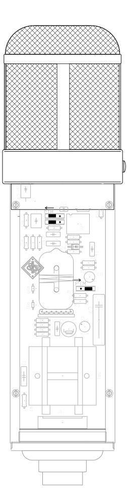
Pure Tube Mode: Jumper shown in Pure Tube Mode Position
